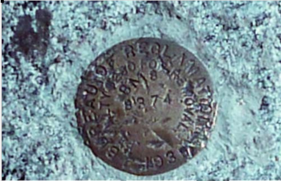
Fig. 12. Bureau of Reclamation survey marker from 1935 placed at the estimated high water line which would be created at the completion of the Colorado-Big Thompson Project. Photo by Steve Batty by permission
